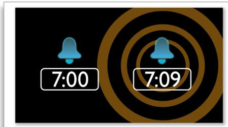
To counter oversleeping, the Philips Clock radio has a snooze feature. Should the alarm ring and you wish to continue sleeping a bit longer, simply press the Repeat Alarm button once and go back to sleep. Nine minutes later the alarm will ring again. You can continue to press the Repeat Alarm button every nine minutes until you turn off the alarm altogether.
